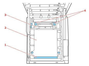
(a) To remove a sheet with its leading edge at the front of the belt (1), carefully lift the sheet from the belt and pull it forwards into the internal drum cavity and withdraw the sheet.
